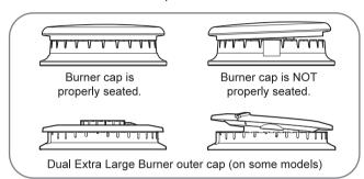
To place the dual extra large burner outer cap properly, make sure the slit in the burner cap is positioned over the assembly guide in the burner head.
