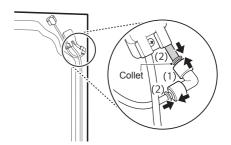
2 Remove the screw (1) from the hinge cover at the top of the refrigerator. Lift the hook (not visible), located at the bottom of the front side of the cover (2) with a flat-head screwdriver.
