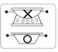
Flames larger than the bottom of the cookware will not result in faster heating of the cookware and could be hazardous.
