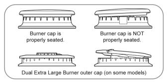
To place the dual extra large burner outer cap properly, make sure the slit in the burner cap is positioned over the assembly guide in the burner head. (LCG3091\*\*, LCG3691\*\* only)
