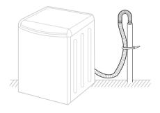
3 If the water valves and drain are built into the wall, fasten the drain hose to one of the water hoses with the tie strap provided (ribbed side on inside).
