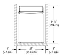
To ensure sufficient clearance for water lines, the drain line and airflow, allow minimum clearances of at least 1 inch (2.5 cm) at the sides and 4 inches (10 cm) behind the unit. Be sure to allow for wall, door. or floor moldings that may increase the required clearances.
