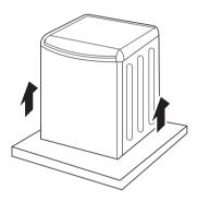
If you must lay the washer down to remove the base packaging materials, always protect the side of the washer and lay it carefully on its side. Do not lay the washer on its front or back.
