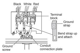
If screws are not tightened securely, it can result in electrical spark and severe personal injury or death.
