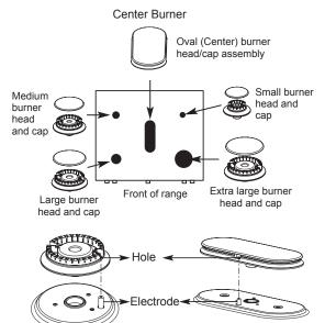
Make sure the hole in the burner head is positioned over the electrode.
