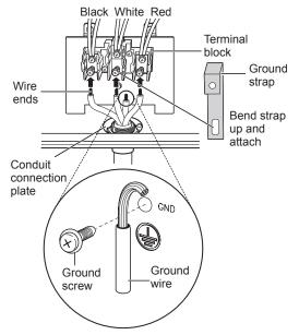
If screws are not tightened securely, it can result in electrical spark and severe personal injury or death.
