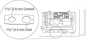
Remove the conduit connection plate
