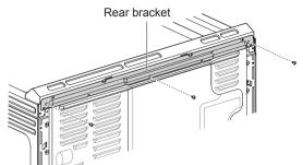
2 Attach the rear bracket and filler assembly as shown, using the three screws removed in step 1.
