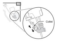
2 Remove the screw (1) from the hinge cover at the top of the refrigerator. Lift the hook (not visible), located at the bottom of the front side of the cover (2) with a flat-head screwdriver.
