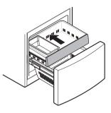
5 Replace the ice bin in the drawer. Insert the Durabase basket in the rail assembly.
