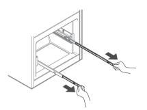
2 Grasp the drawer on each side and hook the drawer supports into the rail tabs located on both sides.
