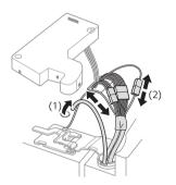
4 Rotate the hinge lever counterclockwise (1). Lift the top hinge (2) free of the hinge lever latch.
