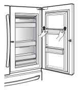
2 To replace the door bins, slide the door bin in above the desired support and push down until it snaps into place.
