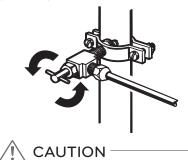
Check to see if leaks occur at the water line connections.
