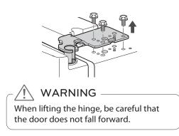
3 Lift the door from the middle hinge pin and remove the door.
