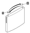
13 Re move the decorative caps on the bottom of the refrigerator housing. You will need these holes for the bottom hinge.
