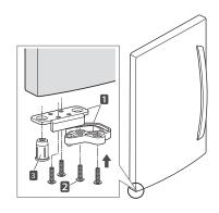
6 Use a ¼ in (6.35 mm) hex socket wrench to loosen the hinge pin 1 and remove. Remove the two bolts 2, the screw 3 and the hinge 4.
