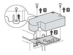
2 Remove the three bolts using a 10mm or 13/32-inch socket wrench and lift off the top hinge. Set parts aside.
