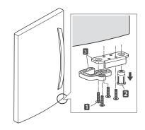
5 Reinstall the hinge pin brackets 1, screws
