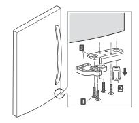
5 Reinstall the hinge pin brackets 1, screws2 and hinge pin insert 3 on the bottom left side of the door.
