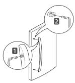
Carefully loosen the plug buttons a with your fingers. The buttons can be unscrewed with the fingers by rotating them counter-clockwise and continuing until they loosen and fall out The buttons were installed without pressure, and for this reason, they can be unscrewed using your index finger, thumb or both. Install the plug buttons s on the left side.
