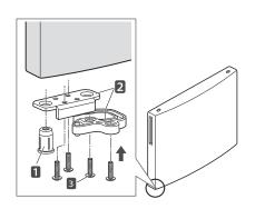
12 On the top part of the door, you will find a cap 1 and a pivot 2. Remove them with a flat head screwdriver and install them on the opposite side ( the cap goes on the right and the pivot on the left).
