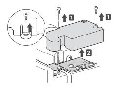
2 Using a13/32 in. or 10 mm socket wrench, remove the three bolts and lift off the top hinge. Set parts aside.
