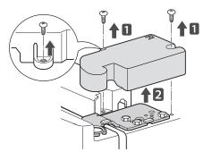
2 Using a 10mm or 13/32 in. socket wrench, remove the three bolts and lift off the top hinge. Set parts aside.
