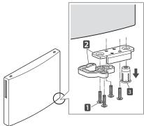
11 Reinstall the hinge pin insert 1, the hinge pin brackets 2 and the screws 3 on the bottom left side of the door.
