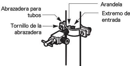
6 ENCAMINE LA TUBERÍA.
