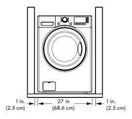
Allow at least  $22^{1}/4$  in. (56.6 cm) in front of the washer to open the door.
