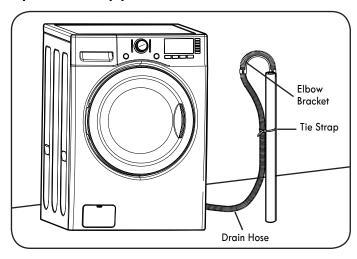
Install the end of the drain hose into the elbow bracket. Do not extend the drain hose more than 4 inches (10 cm) past the end of the elbow bracket. Use a tie strap to secure the drain hose in place.
