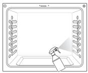
Spray or pour the remaining water onto the bottom center of the oven cavity. The indentation on the oven bottom should be fully covered to submerge all soils. Add water if necessary.
