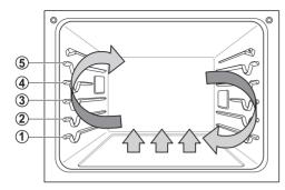
The convection system uses a fan to circulate the heat evenly within the oven. Improved heat distribution allows for even cooking and excellent results while cooking with single or multiple racks.
