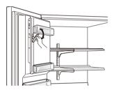
To remove the in-door ice bin, grip the front handle, slightly lift the lower part, and slowly pull out the bin as shown.
