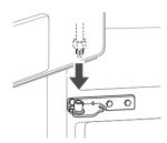
2 Fit the hinge (1) over the hinge lever latch and slot it into place. Rotate the lever clockwise (2) and fasten the hinge.
