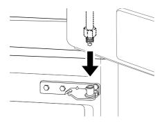
2 Fit the hinge 1 over the hinge lever latch 2 and slot it into place. Rotate the lever 3 counterclockwise to secure the hinge.
