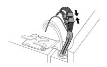
4 Push the water supply lines into the hole on the top case and pull it through the backplate.
