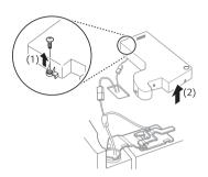
2 Disconnect all the wire harnesses (1). Unscrew the ground wire (2).
