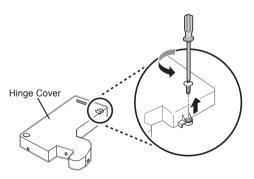
2 Disconnect all the wire harnesses (1). Unscrew the ground wire (2).
