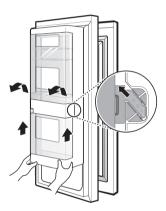
2 To replace the case, line up the tabs on the case with the slots on the door and push down until it snaps into place.
