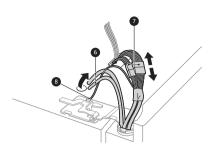
3 Rotate the hinge lever 9 counterclockwise. Lift the top hinge 10 free of the hinge lever latch 10.
