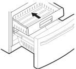
5 Replace the ice bin in the drawer. Insert the Durabase basket in the rail assembly.
