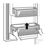
To replace the bin, slide it in above the desired support and push down until it snaps into place.
