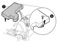
**3** Remove the cover and pull out the tube **3**. Disconnect all wire harnesses **9**. Unscrew the ground wire **10**.
