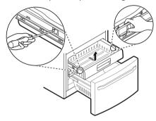
4 Remove the Durabase basket from the rails. Remove the screws from the rails at both ends.
