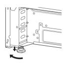
Use a level to check your adjustments. Place the level diagonally on the oven rack, and check each direction for level
