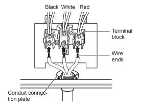
If screws are not tightened securely, it can result in electrical spark and severe personal injury or death.
