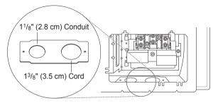
Remove the Conduit connection plate
