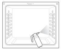
Spray or pour the remaining 1 cup (8 oz or 250 ml) of water onto the bottom center of the oven cavity. The indentation on the oven bottom should be fully covered to submerge all soils. Add water if necessary.
