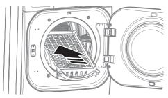
2. Make sure it is seated evenly on the edge of the inner door rim and resting flat on the inside of the dryer.
