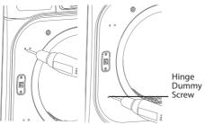
4. Remove two screws and disassembly Latch.
