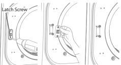
5. Hold on the hinge while remove 2 screws of hinge (to prevent door dropping).
