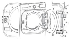
3. Remove four dummy screws by driver.
