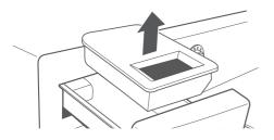
3. Fill the steam feeder just to the filter screen.
