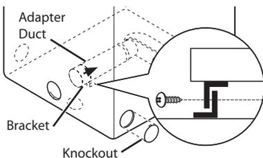
3. Preassemble a 4 inches (10.2 cm) elbow to the next 4-inches (10.2 cm) duct section, and secure all joints with duct tape. Be sure that the male end of the elbow faces AWAY from the dryer. Insert the elbow/duct assembly through the side opening and press it onto the adapter duct. Secure in place with duct tape. Be sure that the male end of the duct protrudes 1½ inches (3.8 cm) to connect the remaining ductwork. Attach cover plate to the back of the dryer with included screw.
