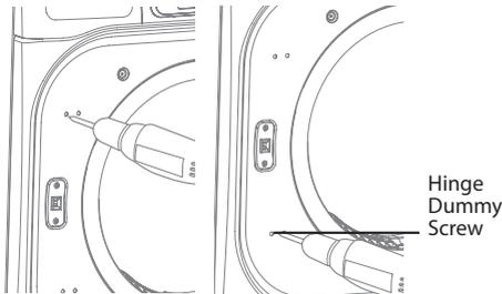
4. Remove two screws and disassembly Latch.
