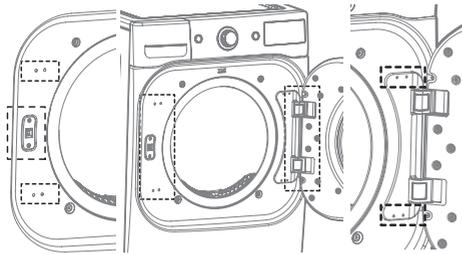
3. Remove four dummy screws by driver.
