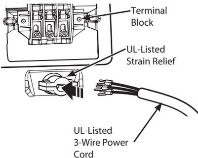
• Use a **30 A, 240 V, UL-listed power cord with #10 AWG-minimum copper** conductor and closed loop or forked terminals with upturned ends.
