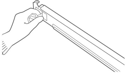
2. Fit the side bracket to the side of the washer top as shown in the above illustration. Firmly press the adhesive area of the bracket to the washer surface. Secure the side bracket to the washer with a screw on the back side of the bracket. Repeat steps 1 and 2 to attach the other side bracket.
