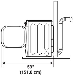
If the duct isn't installed in the wall.
