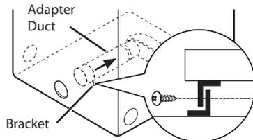
3. Insert the 4 inches (10.2 cm) elbow through the rear opening and press it onto the adapter duct. Be sure that the male end of the elbow faces down through hole in the bottom of the dryer. Secure in place with duct tape. Attach the cover plate to the back of the dryer with included screw.
