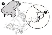
3 Remove the cover and pull out the tube h. Disconnect all wire harnesses i. Unscrew the ground wire j.
