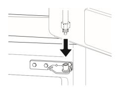
2 Fit the hinge a over the hinge lever latch b and slot it into place. Rotate the lever c counterclockwise to secure the hinge.
