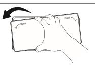
2 Remove the filter from the inside of the cover by pressing the side of the filter in and pulling the center out.
