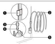
a Tubing Clamp b ¼ in. Tubing c
