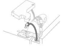
5 Hold the water supply connection and gently push in the collet d to connect the water supply line as shown. Insert the tube at least 5/8 inch (15 mm) into the connector. Insert the clip on the joint to fasten the tube in place.
