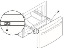
4 Insert the drawer into the frame, and push the drawer back until it clicks into place.
