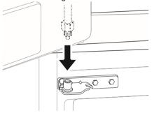
2 Fit the hinge a over the hinge lever latch b and slot it into place. Rotate the lever c clockwise and fasten the hinge.
