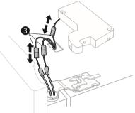
**3** Rotate the hinge lever d clockwise. Lift the top hinge e free of the hinge lever latch f.
