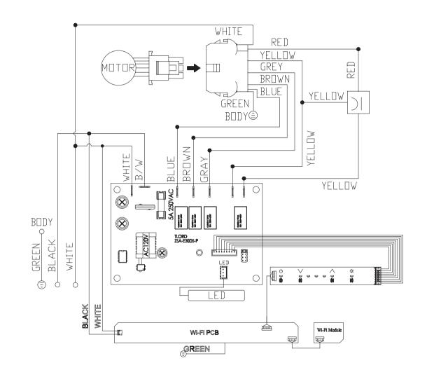
REMARKS:CONDENSER 12.5+12.5uF 250VAC FIT AC120V 60Hz
