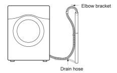
3 Use a tie strap to secure the drain hose in place.
