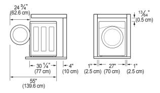
To ensure sufficient clearance for water lines, the drain line and airflow, allow minimum clearances of at least 1 inch (2.5 cm) at the sides and 4 inches (10 cm) behind the unit. Be sure to allow for wall, door, or floor moldings that may increase the required clearances.
