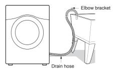
3 Use a tie strap to secure the drain hose in place.
