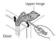
**5** Lift the upper hinge fixed between the appliance and the appliance door and then remove it.
