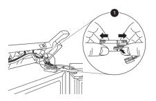
**3** Remove the hinge lever by tapping the end of it toward the outside edge of the cabinet.
