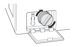
Close the drain pump filter cover.
