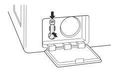
Insert the drain pump filter.
