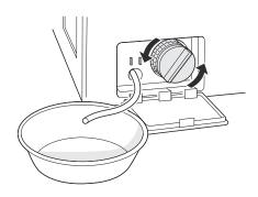
Clean the pump filter and opening.
