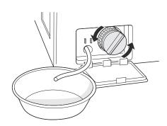
**5** Clean the pump filter and opening.
