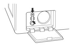
Insert the drain pump filter.
