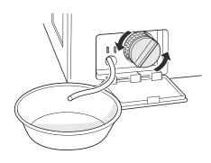
**5** Clean the pump filter and opening.
