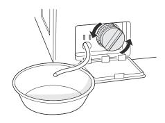
Clean the pump filter and opening.
