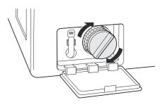
Close the drain pump filter cover.
