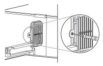
Press on the hooks at the air filter and then take it out.
