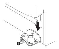
2 Fit the hinge 2 over the hinge lever latch 3 and slot it into place. Rotate the lever 4 counterclockwise to secure the hinge.
