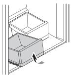
5 Insert the cover into the refrigerator with both hands and lower it onto the guides.
