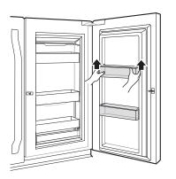
To replace the door bins, slide the door bin in above the desired support and push down until it snaps into place.
