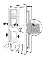
Lift the front of the cover up with both hands until it detaches from the back wall of the cabinet, then pull it out.
