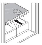
Line up the tabs on the Door-in-Door case with the slots on the door and push down until it snaps into place.
