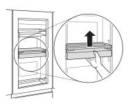
To lower the bin, press the side levers up at thesame time and move the bin down until it clicks into place.
