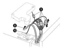
Rotate the hinge lever **1** counterclockwise. Lift the top hinge **1** free of the hinge lever latch 📵.
