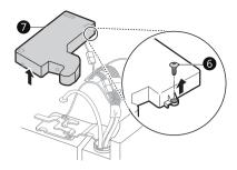
Remove the cover and pull out the tube **8**. Disconnect all wire harnesses **9**. Unscrew the ground wire **①**.
