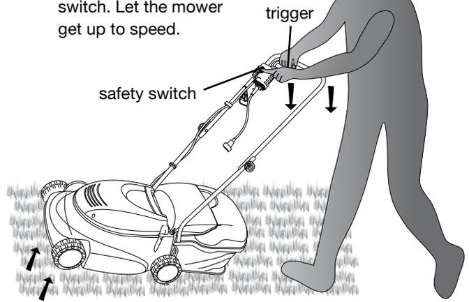
**Step 3:** Slowly lower the lawn mower so the front wheel is on the ground and start mowing.
