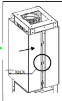
Slide upper "slot" chimney (USC) into place connecting the 6 "C" lock — 3 on each side.
