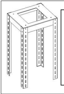
Attach the multi-hole brackets (P2) to the outside 4 corners of the ceiling brackets (P1).
