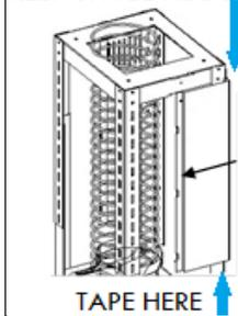
Slide upper "hook" chimney (UHC) in, leave about 1" from the ceiling. Use tape to hold it up from falling down if you don't have any helper to hold it.
