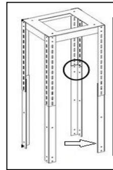
Attach lower chimney bracket (P3) vertically to the inside of the 4 multi-hole brackets (P2) installed in the previous step. Make sure to adjust to its "TOTAL BRACKET LENGTH". Refer to dimension table page 4.
