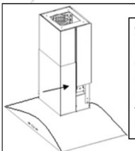
Set the lower "HOOK" chimney piece into place so it drops into the top of the hood.
