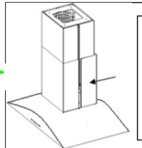
Carefully slide and drop lower "SLOT" chimney into place. Make sure SLOT and HOOK are snapped.
