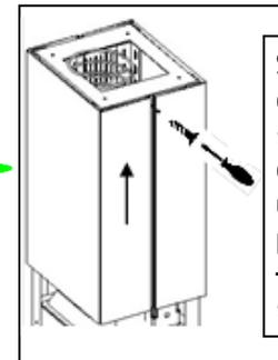
Slide the entire chimney up and secure with the ceiling bracket using the 2 provided bolts — 1 on each side.
