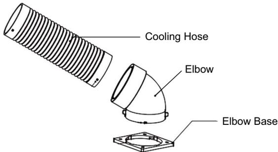
Attach the Elbow to the Elbow Base by turning counter-clockwise. When firmly installed there will be a click.
