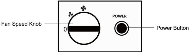
Press the Power Button to turn the OAC on.
