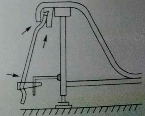
d. The distance between the edge of bathtub and wall is about 0.5cm, the aperture should be filled up and fixed by glass cement.
