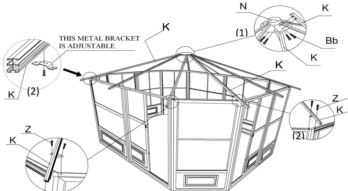
**Note:** Do not tighten the bolts right away as you may have to adjust the angle when inserting the PC roof panels.
