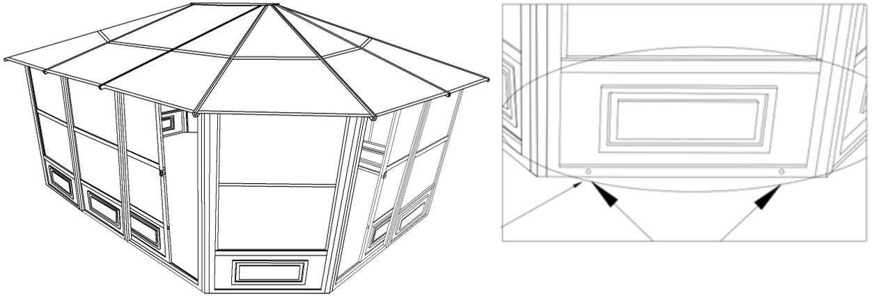
On the outside face, it is suggested to drill holes at the bottom end of the panels to permit drainage when installing on Concrete floor
