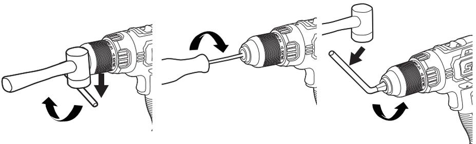
**NOTICE:** The chuck screw has left-handed threads.
