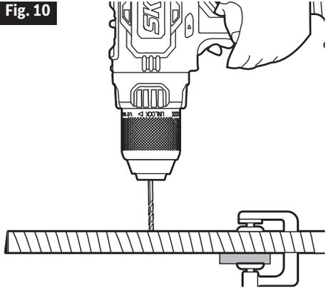
h. If the bit jams in the workpiece or if the drill driver stalls, stop the tool immediately. Remove the bit from the workpiece and determine the reason for jamming.
