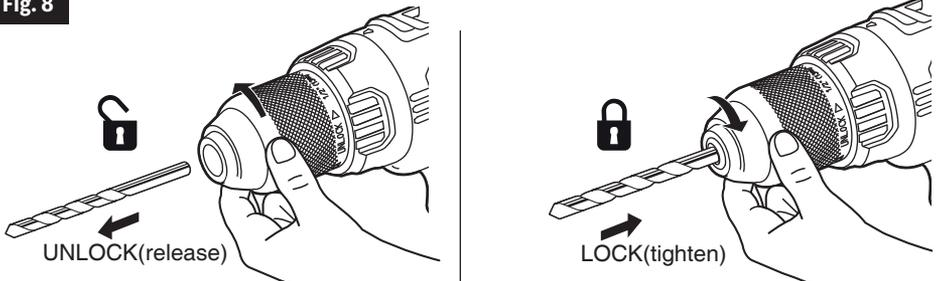
**⚠ WARNING** Use protective gloves when removing the bit from the tool, or first allow the bit to cool down. The bit may be hot after prolonged use.
