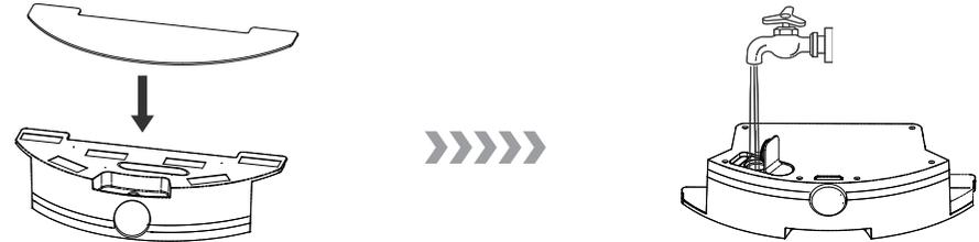
2. Press the dustbin release button, take out the dustbin, and replace it with the water tank.
