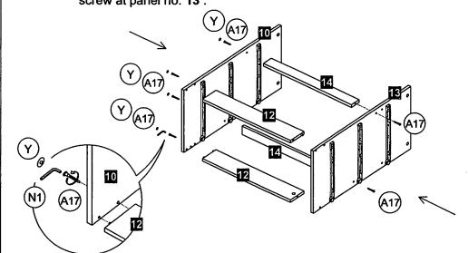
STEP 8 Insert the Mini Fix Double Ended Bolt (F3) at below holes at panel no. 13 & lock with Mini Fix Cam (F3) at both side panel no. 12. Use Allen Key (N1) to tighten the Crosshead Screw 6.3 x 40mm (A17) & button the screw head with Crosshead Cover (Y) except Crosshead Screw (A17) at panel no. 13, (A17)3rd Lock 2nd Insert (F3) **Right Position** 9 (F3) 3rd Lock 1st Insert **Double Ended Bolt**
