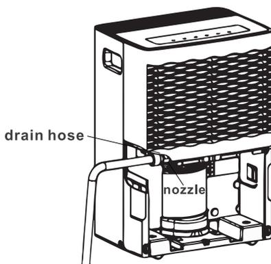
Step 2: Position the gravity drain hose into the floor drain or other water receptacle. Ensure that the gravity drain hose is directed downwards. If the drain hose is directed upwards or horizontally, water will not exit the drain hose and instead will collect in the drain bucket.
