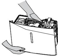
Step 3: After emptying, replace the bucket in dehumidifier following the arrow direction below
