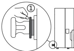
Step 2: While depressing the gray plastic area, remove the green drain plug.
