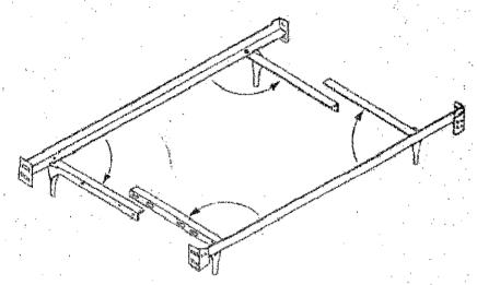
2. Insert the shoulder rivets into the keyhole slots for either the twin or full setting and pull apart to hold in place.
