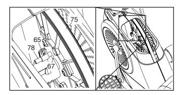
Next, rotate the Pulley (75) until a Magnet (67) is aligned with the Reed Switch (78). Slide the Reed Switch slightly toward or away from the Magnet. Then, retighten the M4 x 12mm Washer Head Screw (65).
