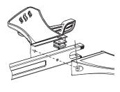
**2** Align the holes on the right and left platforms with the holes on the frame.
