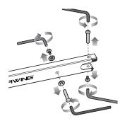
1 Using two (2) 5 mm Allen wrenches, remove the two coupling bolts from the frame.
