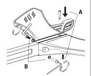
**3** Re-insert coupling bolt (A) first, then re-insert coupling bolt (B). Tighten using two (2) 5 mm Allen wrenches.
