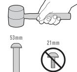
Note: If necessary, carefully tap the coupling bolt with a rubber mallet until it is all the way through the other side of the frame.
