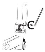
2 With the front wheel pointed straight ahead, the handlebars square to the front wheel and the Razor logo facing the front, use a 5 mm Allen wrench to tighten the two (2) bolts on the collar clamp. The collar clamp is properly tightened when the handlebars cannot be twisted out of alignment with the front wheel.
