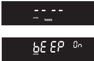
Figure 13: Display changes from dashes to show controls set for audible operation
