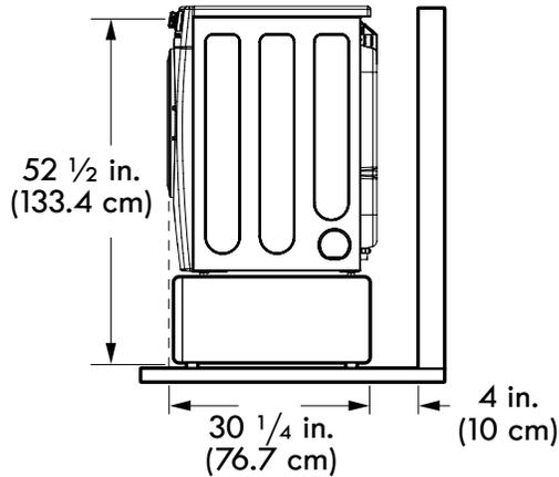
Required Dimensions for Installation with Stacking Kit
