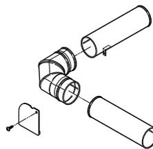
Use the side vent kit for venting directly to either side or to the bottom. Gas dryers can only vent to the left.
