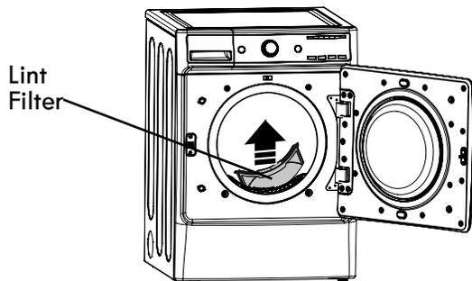
ALWAYS make sure the lint filter is clean before every cycle. The Check Lint Filter Light on the control panel will blink before every cycle to remind you.
