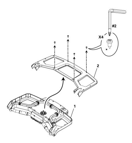
5. Connect the I/O Cables and Attach the Console to Frame Assembly Note: Do not crimp the Cables.
