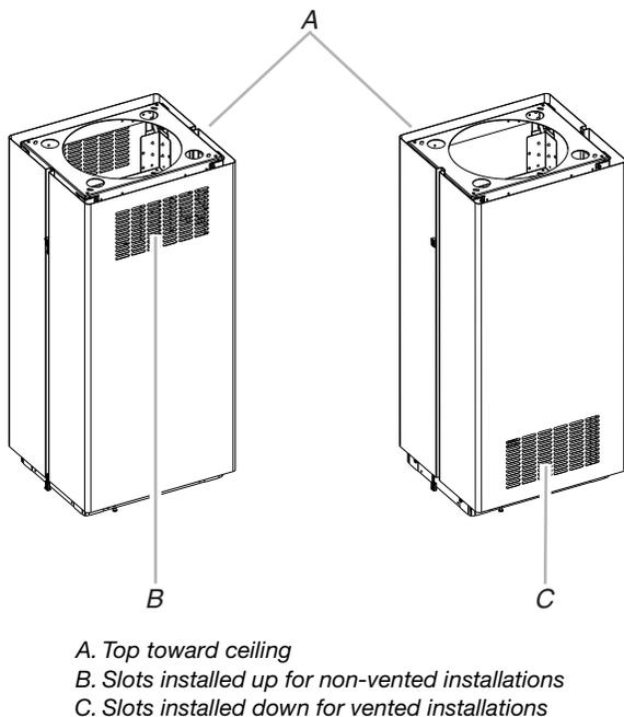
3. Slide the upper duct covers up the frame to the ceiling and secure to the upper horizontal support with 2 - 3.5 x 6.5 mm screws.
