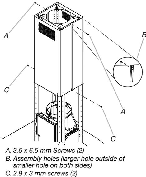
**NOTE:** For non-vented (recirculating) installation, the slotted holes in the upper duct covers will be visible when assembled. For vented installations, the slotted holes will be hidden down inside the lower duct covers.
