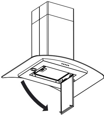
2. Remove each filter by pulling the spring release handle and then pulling down the filter.
