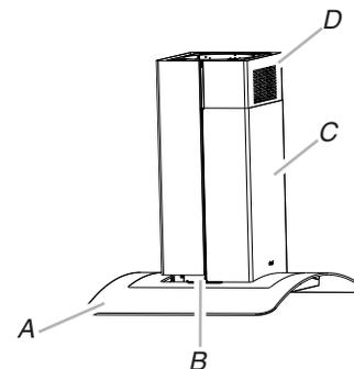
6. Install the lower duct cover (rear) to the range hood canopy. Spread the lower duct cover opening slightly and position it over the upper duct cover. Set the lower duct cover in place. Position so the flanges of the lower duct cover set into the flanges of the upper duct cover. Make sure the front and rear lower duct covers mate properly.
