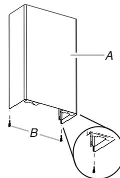
5. Install the lower duct cover (front) to the range hood canopy. Spread the lower duct cover opening slightly and position it over the upper duct cover. Set the lower duct cover in place. Position so the flanges of the lower duct cover set into the flanges of the upper duct covers.
