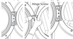
Insert the latch on the right side and install the latch screws.
