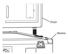
4. Insert the front rail between the bottom of the dryer and the top of the washer. Push the front rail toward the back of the washer until it comes in contact with the side rail stoppers.
