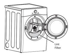
To clean, open the dryer door and pull the lint filter straight up. Then:
