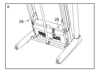
Lower the treadmill (see HOW TO LOWER THE TREADMILL FOR USE on page 24). Remove the five #8 x 3/4" Screws (10). Carefully raise the ends of the Left and Right Foot Rail Covers (49, 73) to remove two of the Screws. Then, carefully remove the Motor Hood (74).
