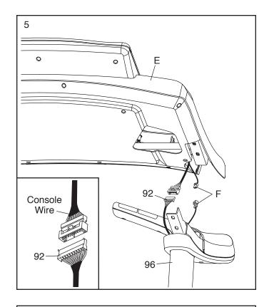
6. With the help of a second person, hold the console assembly (E) near the left handrail assembly (C). Raise the console assembly enough to position the wires (F) so that they will not get pinched as you set the console assembly on the left handrail assembly. Be careful not to pinch any wires.
